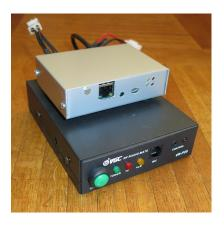
NPR (New Packet Radio) is a custom radio protocol, designed to transport bidirectional IP trafic over 430MHz radio links (ham radio). This protocol is optimized for "point to multipoint" topology, with the help of managed-TDMA. Bitrate is up to 500kbps (net, effective bitrate).
