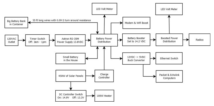
centeralign>VA7FI's setup. The direction of the arrow indicates direction of power.
