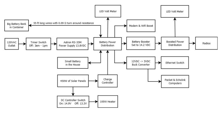
To quantify the voltage drop, I recorded the current draw, the voltage at the house, and the voltage at the container during six short transmissions at different power levels:
