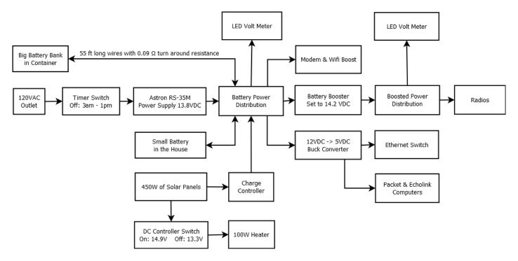
To quantify the voltage drop, I recorded the current draw, the voltage at the house, and the voltage at the container during six short transmissions at different power levels:
