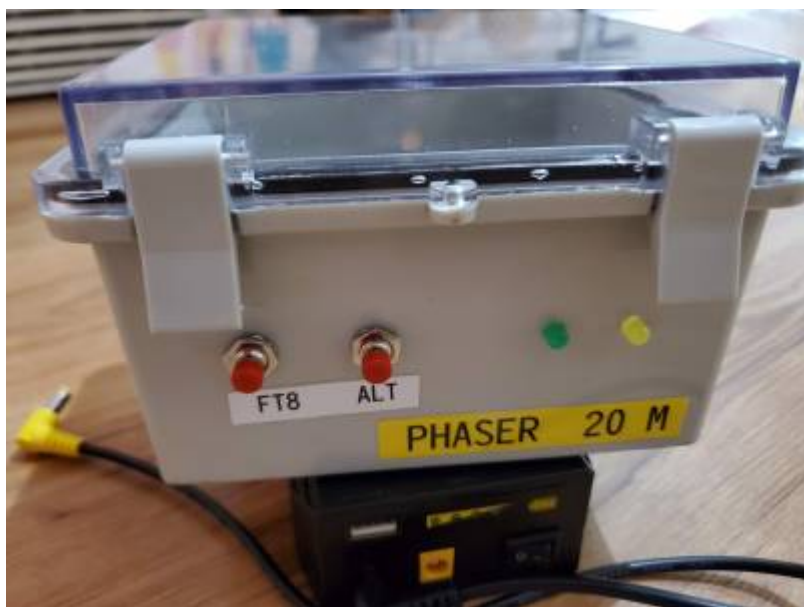
Installed in the case which has a clear lid so the board is visible with the lid closed, the power supply is a TalentCell Model YB1208300-USB 100 watt hour which seems to work well with it for portable operation.
