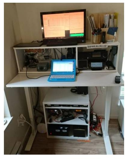
Here's a closeup of the radio cubby. The ID-5100 microphone cord is connecting into an ethernet patch cord to extend it to the radio. On the left, there's a small A/B audio switch so that I can easily connect my headphones into the 5100 without reaching under the desk.
