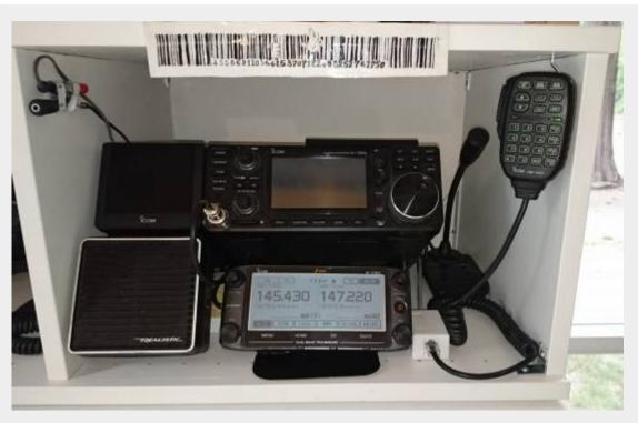
The ID-5100 microphone cord is connected into an Ethernet patch cord to extend it to the radio. On the left, there's a small A/B audio switch so that I can easily connect my headphones into the 5100 without reaching under the desk.
