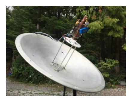
Scott Tilley, VE7TIL, in [Roberts Creek] British Columbia, Canada, received a signal from the NASA Mars Reconnaissance Orbiter (MRO), flying just 274 kilometers (about 170 miles) above the red planet's surface. The signal was an X-band carrier containing no data or telemetry.
