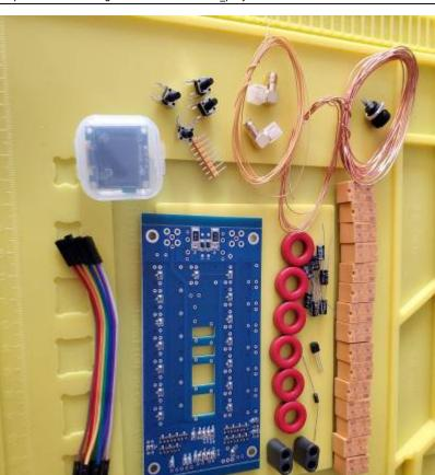
For some reason it came with 3 strips of SMD resistors and 4 PCB mount switches, both of which have nothing to do with the project so that is a bit of a mystery, it also came with an additional binocular ferrite which was an added bonus.
