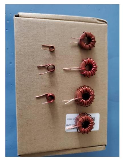
Another note on these ferrites is to make sure you strip or sand off the insulation far enough up so that it is bare on the top side of the board, these are double sided PCBs so the solder needs to flow to the other side to solder to the top pads too.
