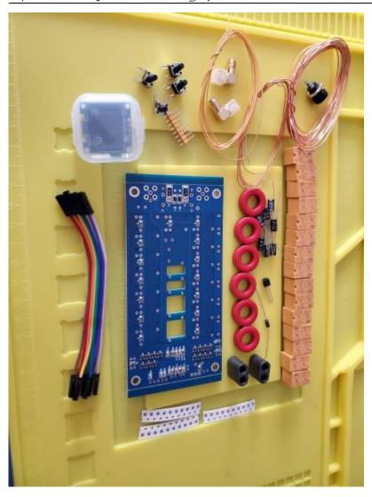
For some reason it came with 3 strips of SMD resistors and 4 PCB mount switches, both of which have nothing to do with the project so that is a bit of a mystery, it also came with an additional binocular ferrite which was an added bonus.
