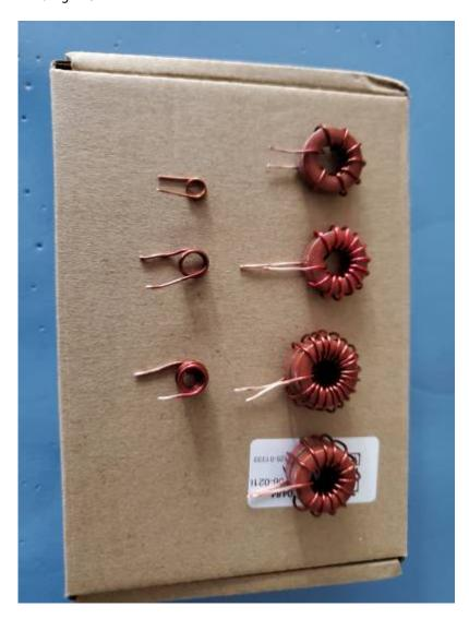
Another note on these ferrites is to make sure you strip or sand off the insulation far enough up so that it is bare on the top side of the board, these are double sided PCBs so the solder needs to flow to the other side to solder to the top pads too.
