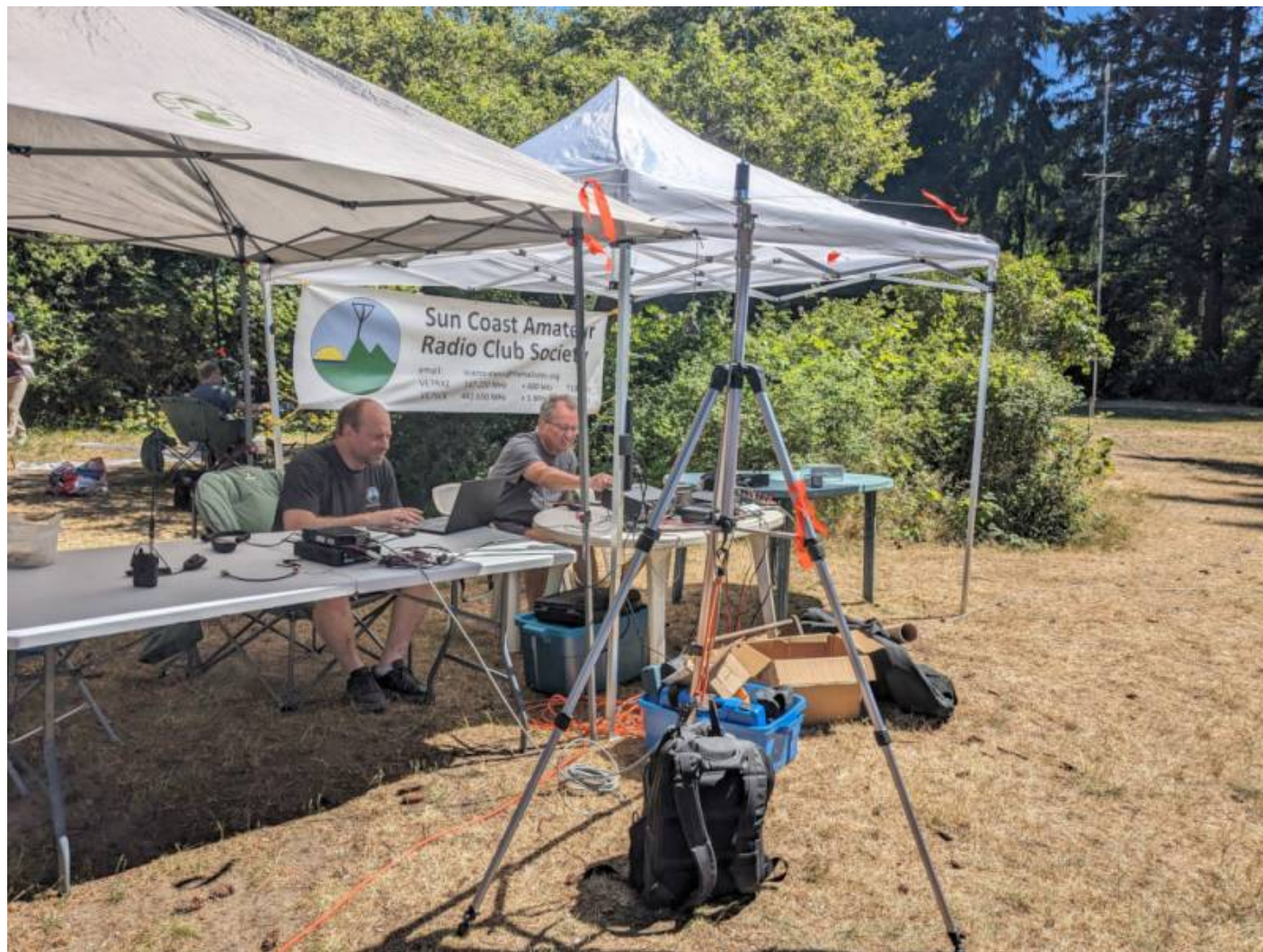
2 metre antenna tripod mounted in the foreground and Hustler multi-band vertical antenna staked in the background
