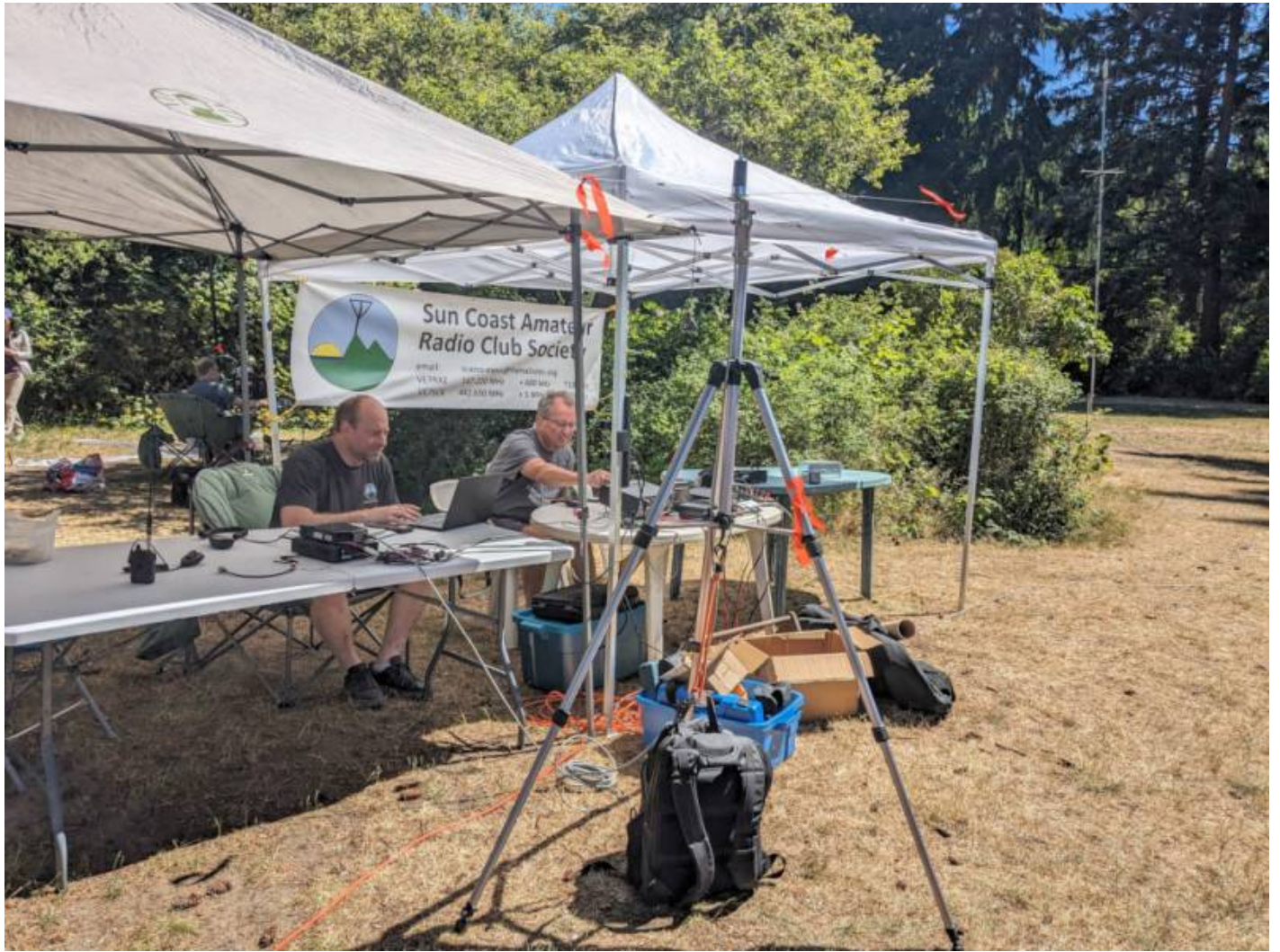
2 metre VHF antenna tripod mounted in the foreground and a Hustler multi-band vertical HF antenna staked in the background
