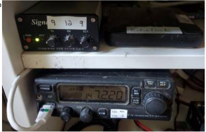
When I first connected it, I had an issue where the volume had to be up and we had to listen to the radio in order for Echolink to work. However, the key was to not use the microphone's audio feed (which keeps the speaker on) but instead use the audio jack at the back (which disables the speaker).
