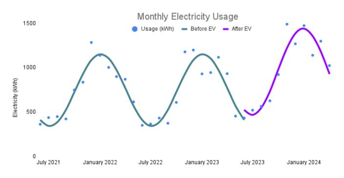
It's interesting to see how the daily consumption after getting the EV is much more scattered than it was before. This is because we don't charge the car everyday so we get spikes when we charge, and regular usage when we don't. To even out the load, we programmed the car to start charging at 11pm. That way, the extra 30A draw doesn't impact our regular usage during the day.
