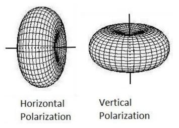
The radiation pattern of a dipole looks like a doughnut, so it makes sense that for a vertically polarized antenna, the "quietest" spots would be right above and below.
