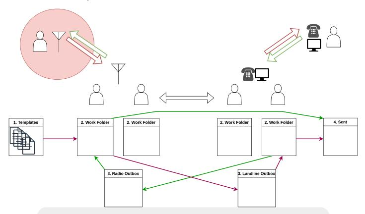
**Scenario**: A disaster zone (circled in red) only has access to radio comms, and various people check in to a net to pass traffic to the wider world. The net controllers are outside the disaster zone and have access to phones and the internet.
