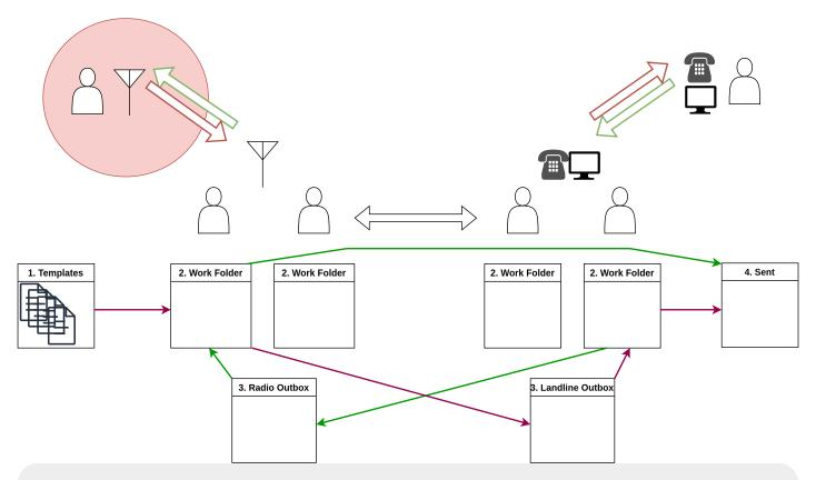
**Scenario**: A disaster zone (circled in red) only has access to radio comms, and various people check in to a net to pass traffic to the wider world. The net controllers are outside the disaster zone and have access to phones
