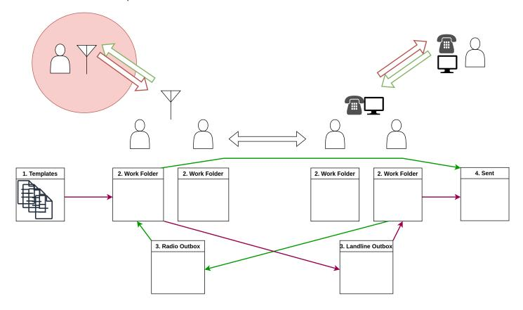
**Scenario**: A disaster zone (circled in red) only has access to radio comms, and various people check in to a net to pass traffic to the wider world. The net controllers are outside the disaster zone and have access to phones and the internet.
