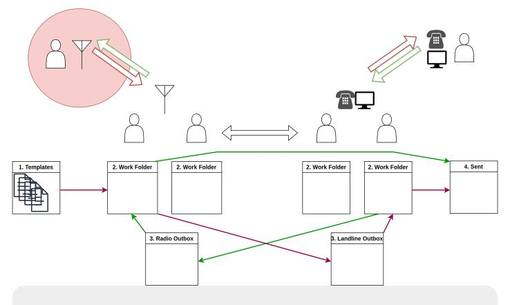
**Scenario**: A disaster zone (circled in red) only has access to radio comms, and various people check in to a net to pass traffic to the wider world. The net controllers are outside the disaster zone and have access to phones
