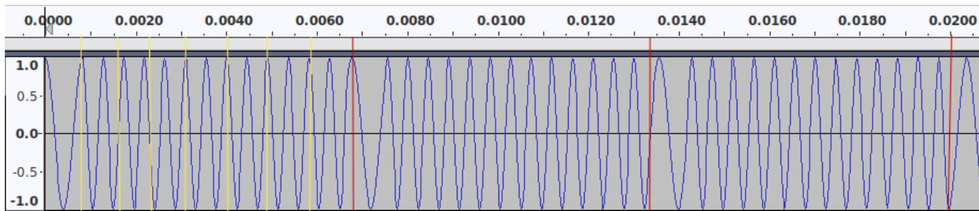
The first half of the transmission contains the same pattern of one long wave (1200 Hz) followed by 12 short waves (2200 Hz) repeated 76 times. I separated these in red. Since each of these sections lasts 1/150th of a second and each note lasts 1/1200th of a second, each section contains 8 notes (separated here in yellow).
