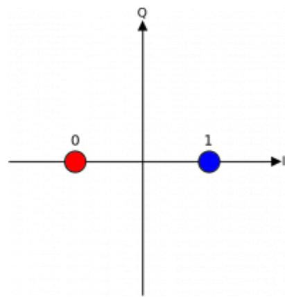
A useful way of representing the different “states” that the waves can be in is using a constellation diagram.<sup>5)</sup> For example, using the Blue and Red waves to encode a message, the constellation diagram would have the two dots on the horizontal axis (one on the right at (1,0) and one on the left at (-1,0)).
