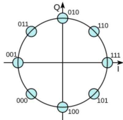
The advantage is that while we might only be able to transmit 1200 notes per second (1200 Baud), the data rate is now triple (3600 bps). That is, each note encodes 3 bits.
