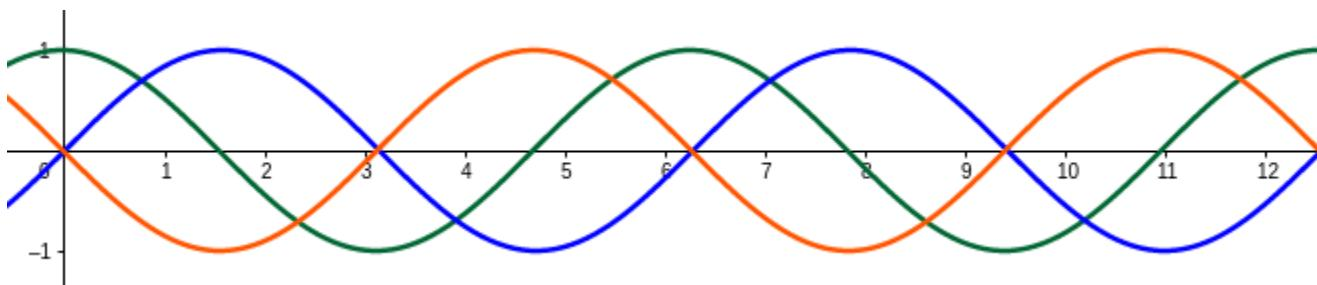
Supposing we use the blue wave as a reference wave, the green wave is 90° out of phase, while the red wave is 180° out of phase. Notice that all three waves have the same frequency (the number of cycles per second) and the same amplitude (the height of the wave), but they start at different points. To the human ear, all three notes would sound exactly the same, but a computer can be made to detect the difference, which means we can use two of those waves to represent different bits.
