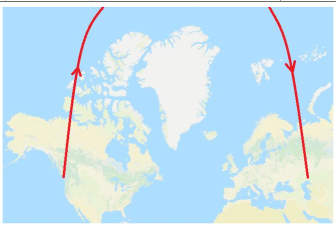
For ham operators, being able to find the shortest straight line between two points on Earth is important because radio waves travel in straight lines. Sure, they bounce, reflect and refract, but they don't just turn left to follow a latitude line. So if you want to know where to point your antenna to reach a specific region, a conventional map won't be much help. Instead, we use what's called an Azimuthal map.
