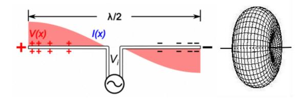
Voila! The antenna we've made is called a *dipole*. Assuming that its length matches the frequency of the current generator (more on this shortly), and that the antenna is high enough above the ground, you've created a radio wave. As electrons move up and down the length of the wires, they create varying electric and magnetic fields that couple together according to Maxwell's Equations and propagate outward in a doughnut shape. Maxwell's Equations are propagated outward in a doughnut shape.
