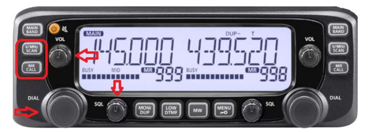
This particular radio is the Icom IC-2730A. The first thing to notice about this radio is that it's actually two radios in one. You can listen to two different frequencies at the same time, with their own independent volumes and dials. So looking at the left side for example, we see...
