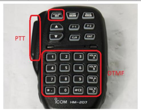
The microphone on this particular radio contains some new buttons, but some that are also on the radio itself like the VFO/MR, VOL and SQL
