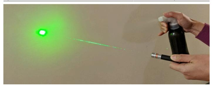
The reason the beam is invisible in the first picture is that all the light from the laser travels toward the wall (and none toward the camera). But in the second picture, the water vapour scatters some of that light in random directions, allowing some of it to reach the camera. There's a subtle point here: light from a regular light bulb also does this. What I mean is this:
