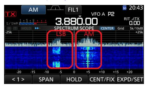
The radio is tuned to 3.880 MHz (where no one is transmitting), but there are two neighbouring conversations going on:
