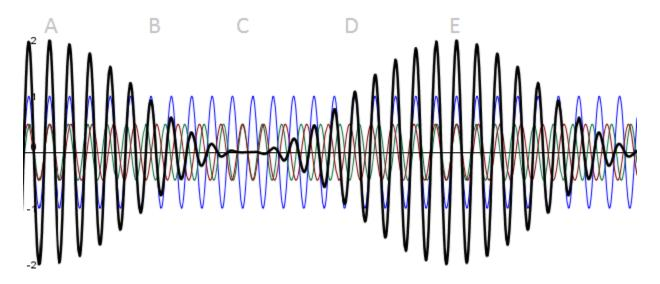
Note that the carrier has a frequency of 200 kHz just like the original carrier, but the two side bands are 10 kHz lower and higher with half of the amplitude. Notice also how the LSB Wave oscillates slower than the Carrier Wave, while the USB Wave oscillates faster.
