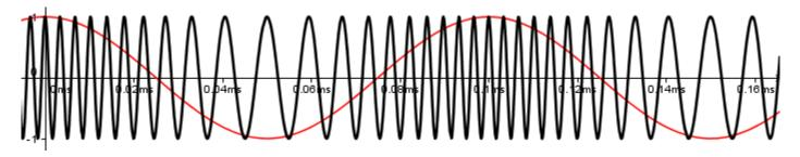
Here, the math is a bit more involved and requires at least  $1^{st}$  year calculus to understand but in a nutshell, if the carrier is  $\s c(t) = \cos(2 pi f_c t)$  and the baseband signal is  $\s s(t)$ , then the FM signal will be:
