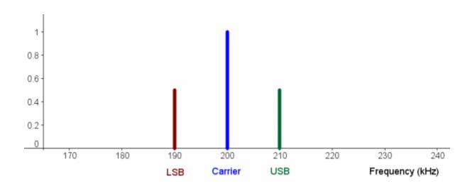
For example, the spectrum of our 10 kHz note transmitted over a 200 kHz carrier would look like this:
