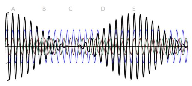
Note that the carrier has a frequency of 200 kHz just like the original carrier, but the two side bands are 10 kHz lower and higher with half of the amplitude. Notice also how the LSB Wave oscillates slower than the Carrier Wave, while the USB Wave oscillates faster.
