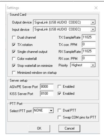
Once the radio, the Signalink, and the Soundmodem are configured, start PinPoint and change these settings:
