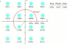
QAM is kind of a mix between PSK and ASK (Amplitude Shift Keying). That is, in addition to being able to vary the phase of the waves (where they start), we can also vary their amplitude (how strong the signal is). In the case of 16-QAM, each note can encode 4 bits. So a 1200 Baud signal has a bit rate of 4800 bps.
