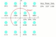
QAM is kind of a mix between PSK and ASK (Amplitude Shift Keying). That is, in addition to being able to vary the phase of the waves (where they start), we can also vary their amplitude (how strong the signal is). In the case of 16-QAM, each note can encode 4 bits. So a 1200 Baud signal has a bit rate of 4800 bps.
