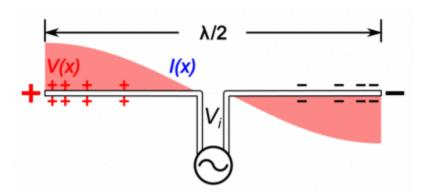
Voila, assuming that the length of the antenna (the two pieces of wires) match the frequency of the current generator, and that the antenna is high enough above the ground, you've created a radio wave.<sup>1)</sup>
