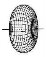
So what happens is that as electrons move up and down the length of the wires, they create a varying electric and magnetic fields that couple together according to Maxwell's Equations and propagate outward in a doughnut
