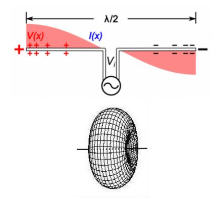
Voila! Assuming that the length of the antenna (the two pieces of wires) match the frequency of the current generator, and that the antenna is high enough above the ground, you've created a radio wave.<sup>1)</sup>
