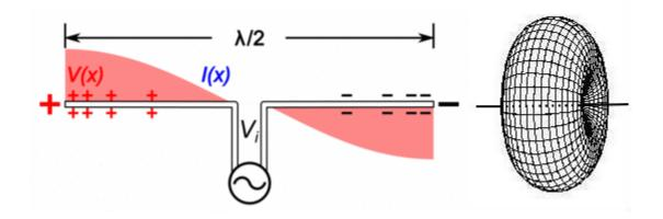
Voila! The antenna we've made is called a *dipole*. Assuming that its length matches the frequency of the current generator (more on this shortly), and that the antenna is high enough above the ground, you've created a radio wave.<sup>1)</sup> As electrons move up and down the length of the wires, they create varying electric and magnetic fields that couple together according to **a** Maxwell's Equations and propagate outward in a doughnut shape.<sup>2)</sup>
