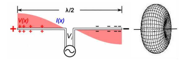
Voila! The antenna we've made is called a *dipole*. Assuming that its length matches the frequency of the current generator (more on this shortly), and that the antenna is high enough above the ground, you've created a radio wave.<sup>1)</sup> As electrons move up and down the length of the wires, they create varying electric and magnetic fields that couple together according to Maxwell's Equations and propagate outward in a doughnut shape.<sup>2)</sup>
