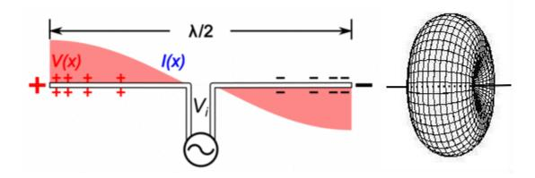
Voila! The antenna we've made is called a *dipole*. Assuming that its length matches the frequency of the current generator (more on this shortly), and that the antenna is high enough above the ground, you've created a radio wave.<sup>1)</sup> As electrons move up and down the length of the wires, they create varying electric and magnetic fields that couple together according to Maxwell's Equations and propagate outward in a doughnut shape.<sup>2)</sup>
