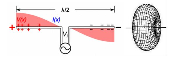
Voila! The antenna we've made is called a *dipole*. Assuming that its length matches the frequency of the current generator (more on this shortly), and that the antenna is high enough above the ground, you've created a radio wave. As electrons move up and down the length of the wires, they create varying electric and magnetic fields that couple together according to Maxwell's Equations and propagate outward in a doughnut shape. Maxwell's Equations are propagate outward in a doughnut shape.
