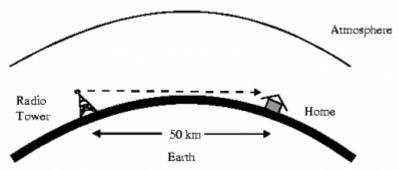
For example, since my antenna is 20m above the ground, and we're up a hill 100m above the water, which I can see from the top of my tree, it means that my antenna can see the to about 45 km in that direction.
