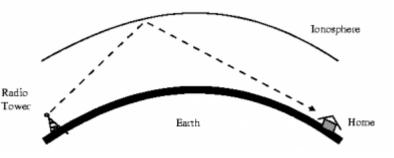
This process uses lonospheric Refraction, which we'll see next.<sup>2)</sup>
