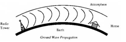
Because it is so low, the radio wave interacts with the ground where it loses some of its energy but also curves toward it. The good news, though, is that even though the radio waves lose energy in the ground, they can go beyond the horizon out to about 200 km.
