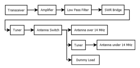
Some of the components shown above may be integrated into one device, and others may be optional. But if all are included, this is how they should be connected.
