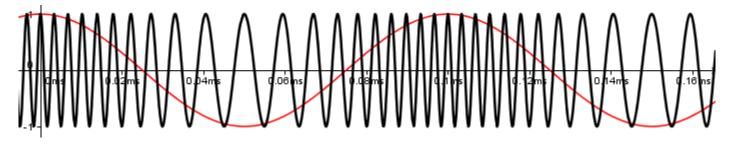
Here, the math is a bit more involved and requires at least  $1^{st}$  year calculus to understand but in a nutshell, if the carrier is \\$\$ c(t) = \cos(2 \pi f c t) \\$\$ and the baseband signal is \\$\$s(t)\\$\$, then the FM signal will be:
