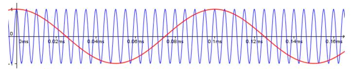
Before we modulate the carrier, we raise the audio signal above zero to get an envelope:
