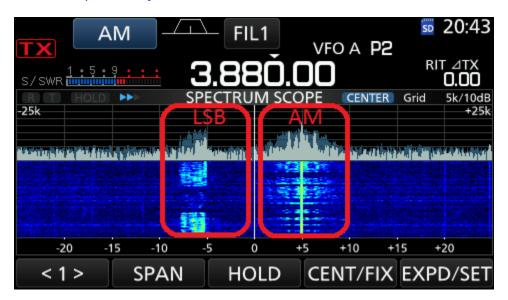
The radio is tuned to 3.880 MHz (where no one is transmitting), but there are two different conversations going on: one at 3.875 MHz using LSB, and another at 3.885 MHz using AM. The scope shows the recent history of the radio signal (called *waterfall*) where the present is at the top and the past at the bottom. Blue represent a low signal and yellow or red represent a high signal. Here are some things to notice:
