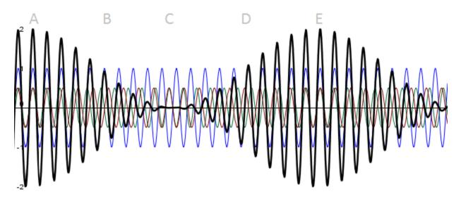
Note that the carrier is at 200 kHz exactly like the original carrier, but that the two side bands are 10 kHz lower and higher with half of the amplitude. Notice how the LSB Wave oscillates slower than the Carrier Wave, while the USB Wave oscillates faster.
