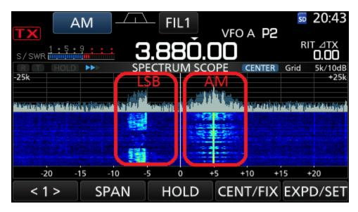
The radio is tuned to 3.880 MHz (where no one is transmitting), but there are two different conversations going on: one at 3.875 MHz using LSB, and another at 3.885 MHz using AM. The scope shows the recent history of the radio signal (called *waterfall*) where the present is at the top and the past at the bottom. Blue represent a low signal and yellow or red represent a high signal. Here are some things to notice:
