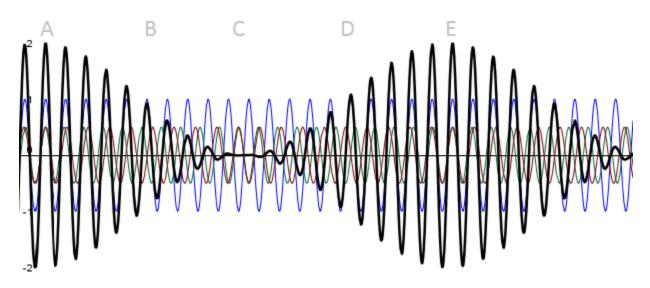
Note that the carrier is at 200 kHz exactly like the original carrier, but that the two side bands are 10 kHz lower and higher with half of the amplitude. Notice how the LSB Wave oscillates slower than the Carrier Wave, while the USB Wave oscillates faster.
