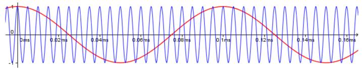
This time, we don't simply multiply the baseband signal to the carrier (as in AM). Instead, we "compress" and "stretch" the carrier (ie, modulate its frequency) based on the baseband signal.
