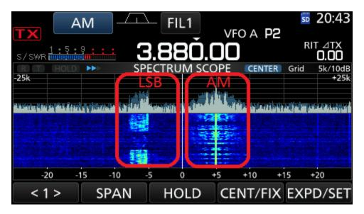
The radio is tuned to 3.880 MHz (where no one is transmitting), but there are two different conversations going on: one at 3.875 MHz using LSB, and another at 3.885 MHz using AM. The scope shows the recent history of the radio signal (called *waterfall*) where the present is at the top and the past at the bottom. Blue represent a weak signal strength and yellow or red represent a strong signal strength. Here are some things to notice:
