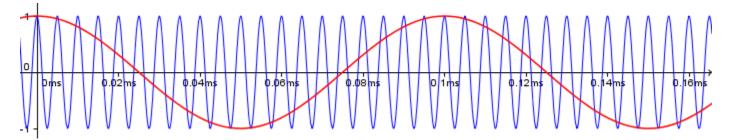
Before we modulate the carrier, we raise the audio signal above zero to get an envelope:
