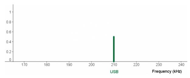
By itself, neither of these transmissions would carry the information we need (that the baseband signal was a 10 kHz note) since it's the difference between the sideband and the carrier that gives us that information. But if the receiver knows that this signal was generated by a transmitter at a frequency of 200 kHz, then the receiver can re-
