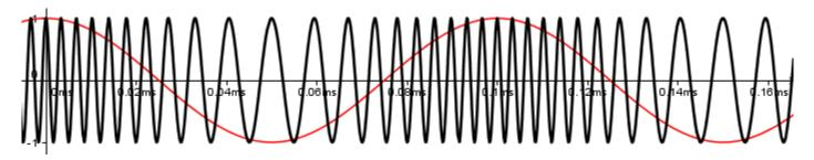
Here, the math is a bit more involved and requires at least 1st year calculus to understand but in a nutshell, if the carrier is <|atex>  $c(t) = cos(2 pi f_c t)$ , and the baseband signal is <|atex>, then the FM signal will be:
