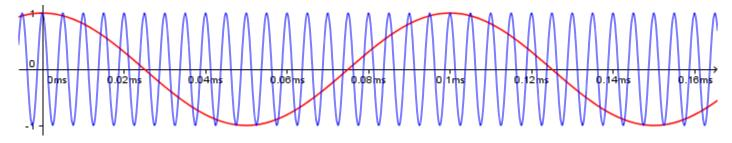
This time, we don't simply multiply the baseband signal to the carrier (as in AM). Instead, we "compress" and "stretch" the carrier (ie, modulate its frequency) based on the baseband signal.
